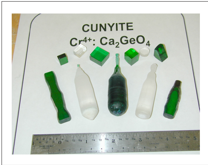
C UNYITE crystals ( \text{Cr}^{4+}:\text{Ca}_2\text{GeO}_4 ) grown by the Czochralski technique.
